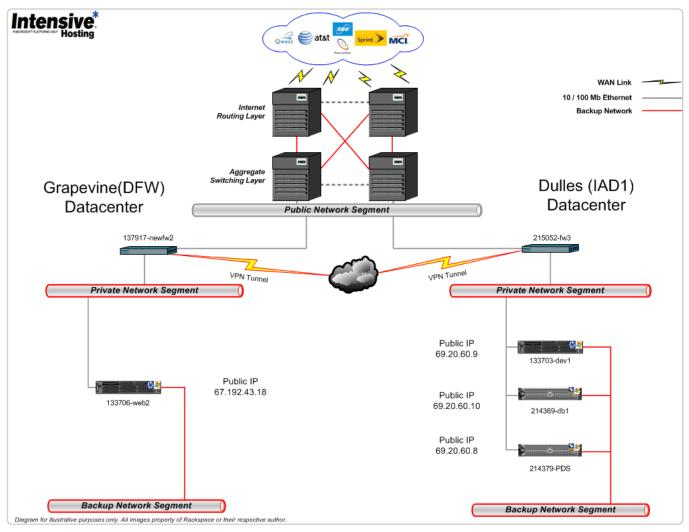
Figure 1: The PDS Network Configuration
