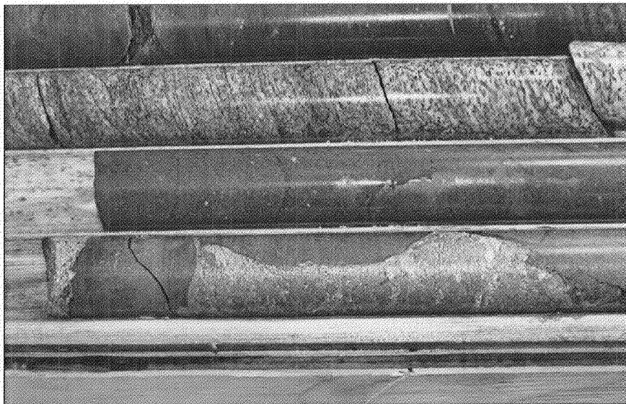
Photo 7. Remobilized massive sulphides (pyrrhotite, pentlandite, chalcopyrite) over 30 centimetres in pyroxenite at 27.10 metres (GA-12-094).
