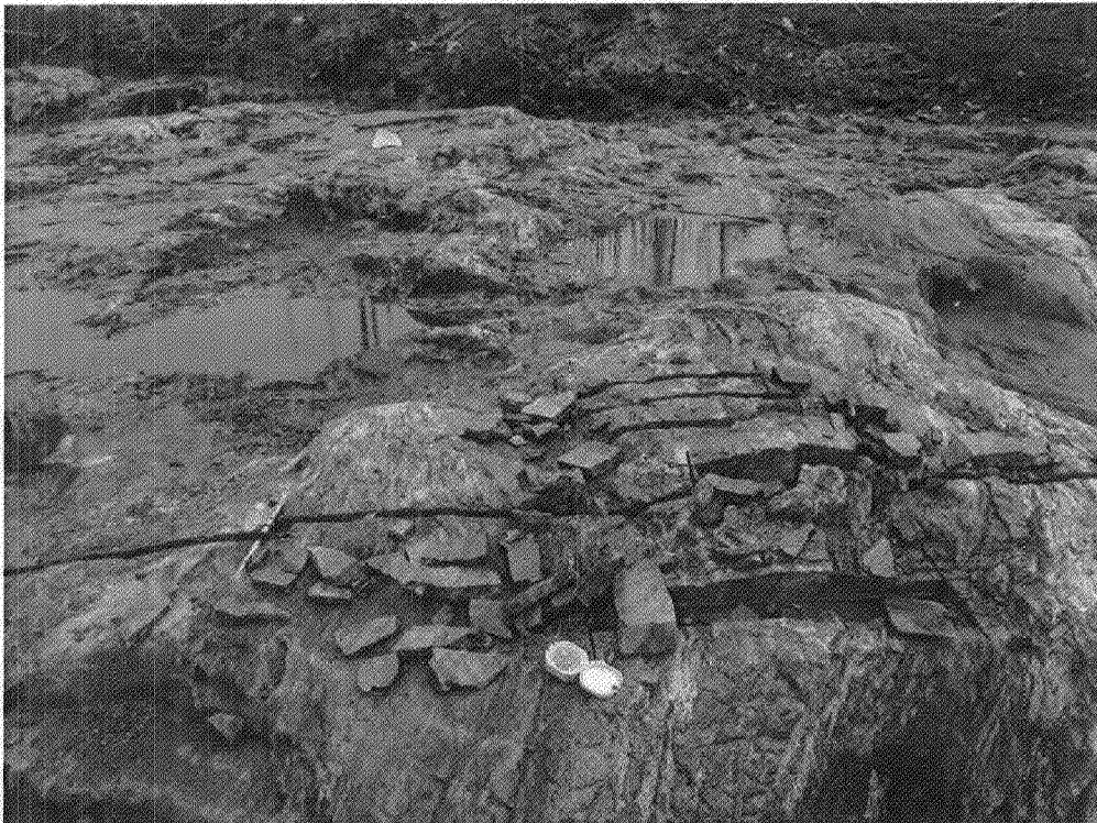
Photo 9 : Mineralized zone in trench WB2012TR031 : 4.69 g/t Au over 5.00 m from 0.00 to 5.00 metres from channel R3. Presence of about forty gold grains in quartz vein and in a wacke highly altered in silica, feldspar, sericite and chlorite.
