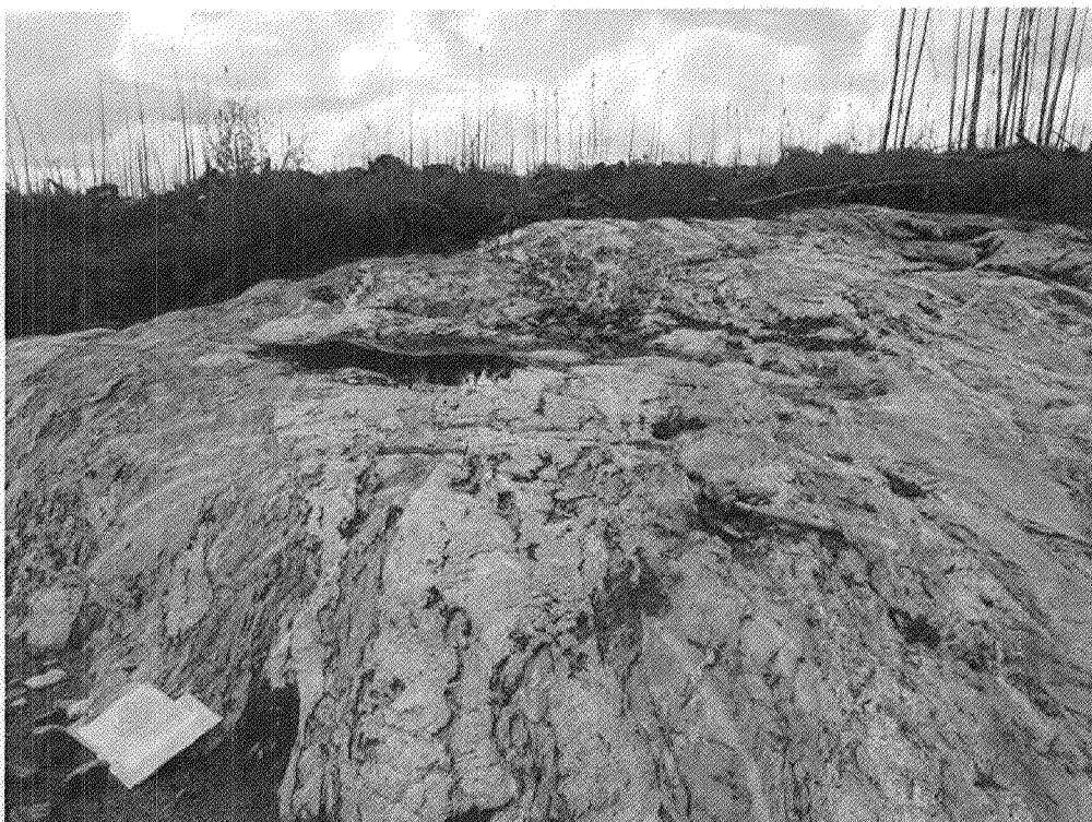
Photo 12: General aspect of trench WB2012TR020 covered by 60% of axial plan quartz veins axial plane, extensional veins and subhorizontal veins.
