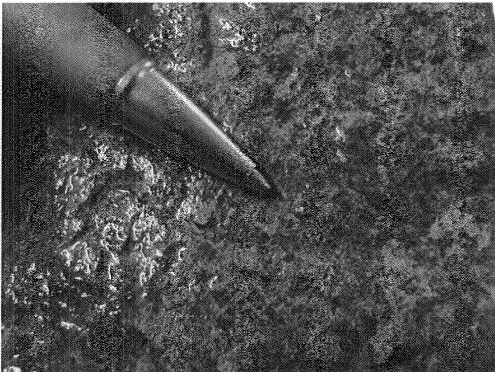
Photo 22 : WB2012TR072 : Visible gold located in a massive coarse-grained wacke that contains 15-20% pervasive hornblende (WISP). The gold was seen only on the surface of the outcrop.
