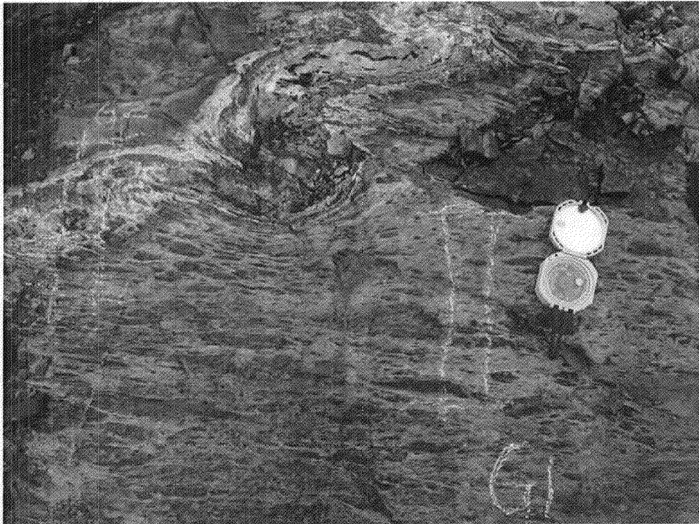
Photo 20 : WB2012TR015 : Decimetric gold-bearing vein with footwall strongly altered to chlorite, feldspar, sericite. Near the vein, the wacke is altered with a banded-fragmented texture as are the walls of the Mustang vein. The vein is folded into an S. About forty visible gold grains were observed in the channels and one was seen on the surface of the wacke (red circle).
