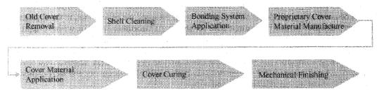
The covering on the rolls used in the paper-making process wear over time and must be periodically replaced for the roll to function properly. Rolls are removed from the paper-making machine and taken to an offsite facility for re-covering. During this time, a spare roll is placed in the machine to enable continuous operations.
