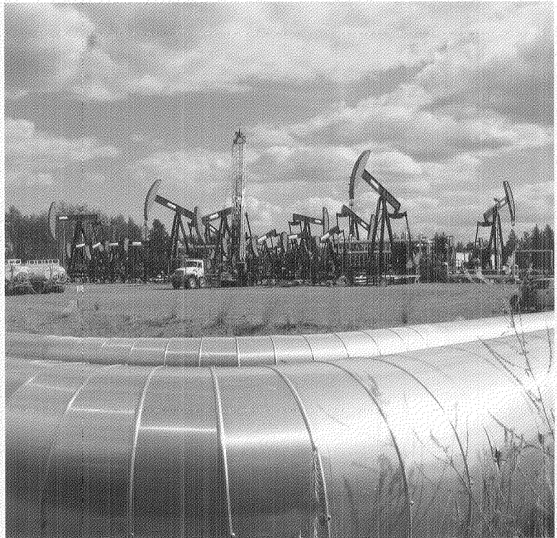
Weatherford's COROD® continuous rod and Ampscot pumping units have been running in Imperial Oil oilfields in Cold Lake, Alberta, for over two decades.
