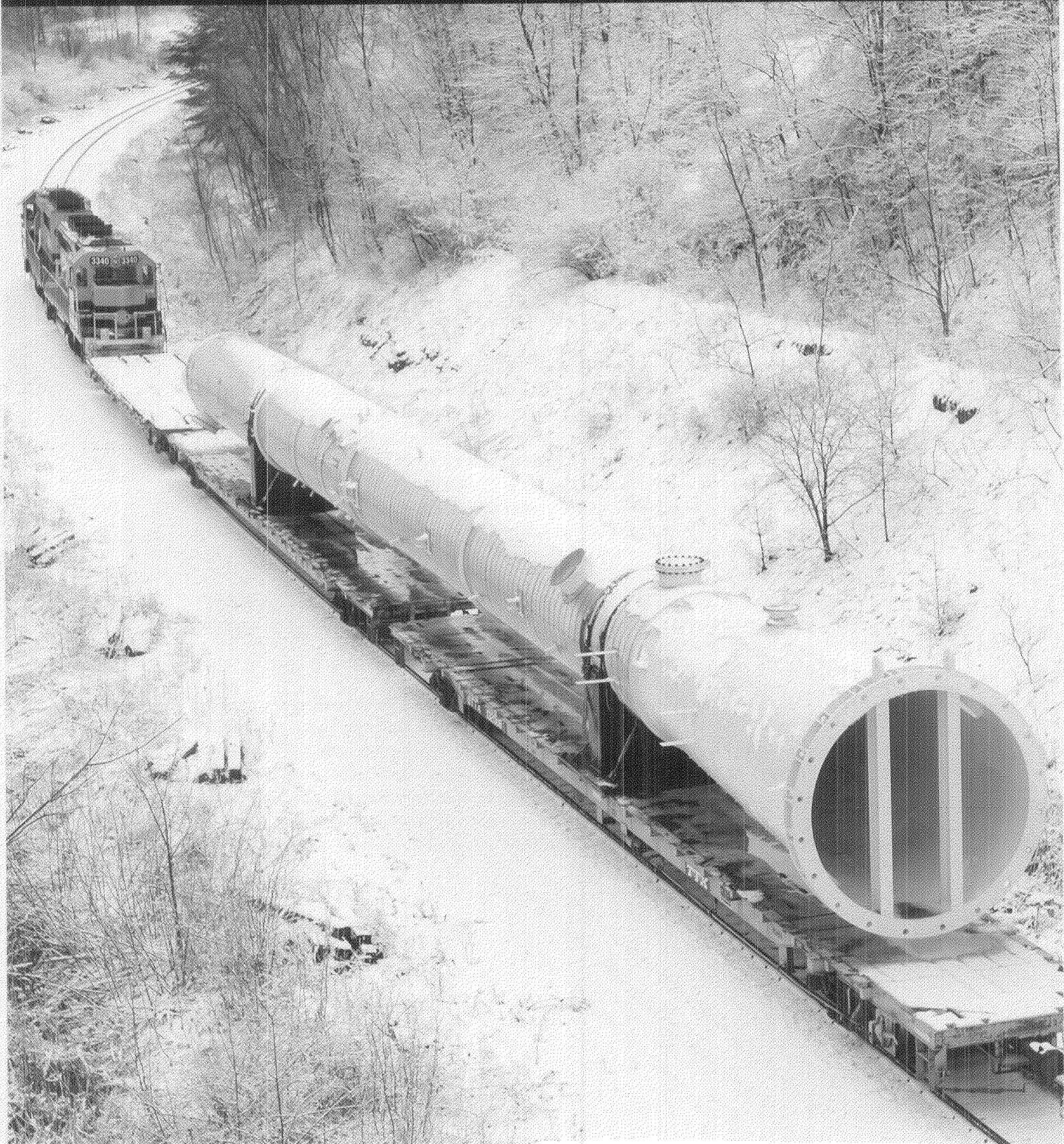
A special train on G&W's Columbus & Ohio River Rail Road (CUOH) transports a 138-foot debutanizer tower for installation at the CUOH-served natural gas liquids (NGLs) processing/fractionation/storage hub being built by Utica East Ohio Midstream, LLC at Scio, Ohio.
