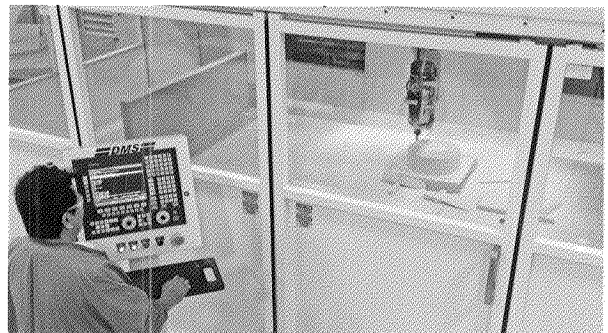
CNC Router cutting a holding fixture for a composite part that will be trimmed on the CNC Router.
