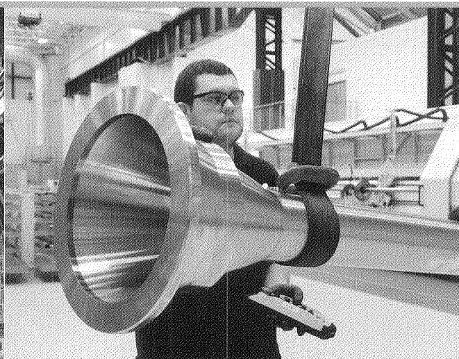
A machined jet engine shaft at our Precision Machining Facility in Sheffield, U.K.
