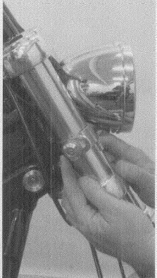
The first step is to test-fit the Memphis Shades fork clamp to find out which slot to use.
