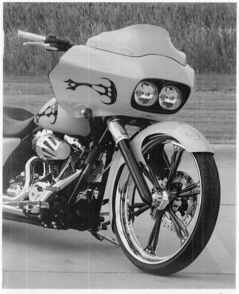
were the cylinder heads, ported and polished by Earl Burley of Burley Performance in Ridgecrest, California. Earl works the old-fashioned way, shaping and polishing the ports by hand. He checks his work with a flow bench, too. For this job he installed 1.9" intake and 1.6" exhaust valves, designing the ports to match the specifications of the Woods 555 cam and Fat Cat exhaust.
