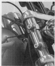
Loosely install the clamps using a 3/16" Allen.
