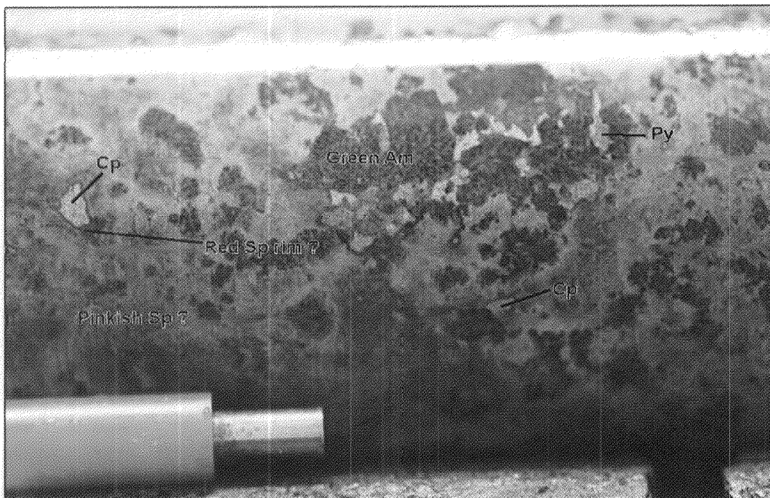
Photo 3: Pinkish-beige sphalerite with chalcopyrite and green amphibole outlined @ 790.6m in CN-12-257.
