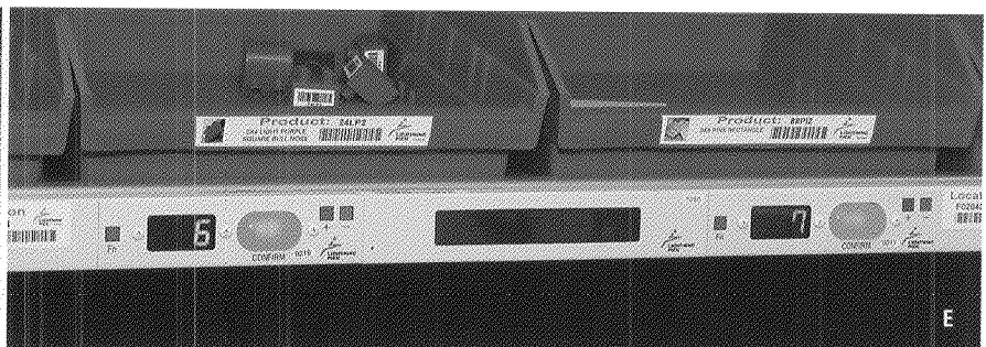
(D and E) Pick-To-Light Systems – Light-directed order fulfillment systems use light indicator modules mounted to shelving or other storage locations that indicate when a product is needed from a particular location.
