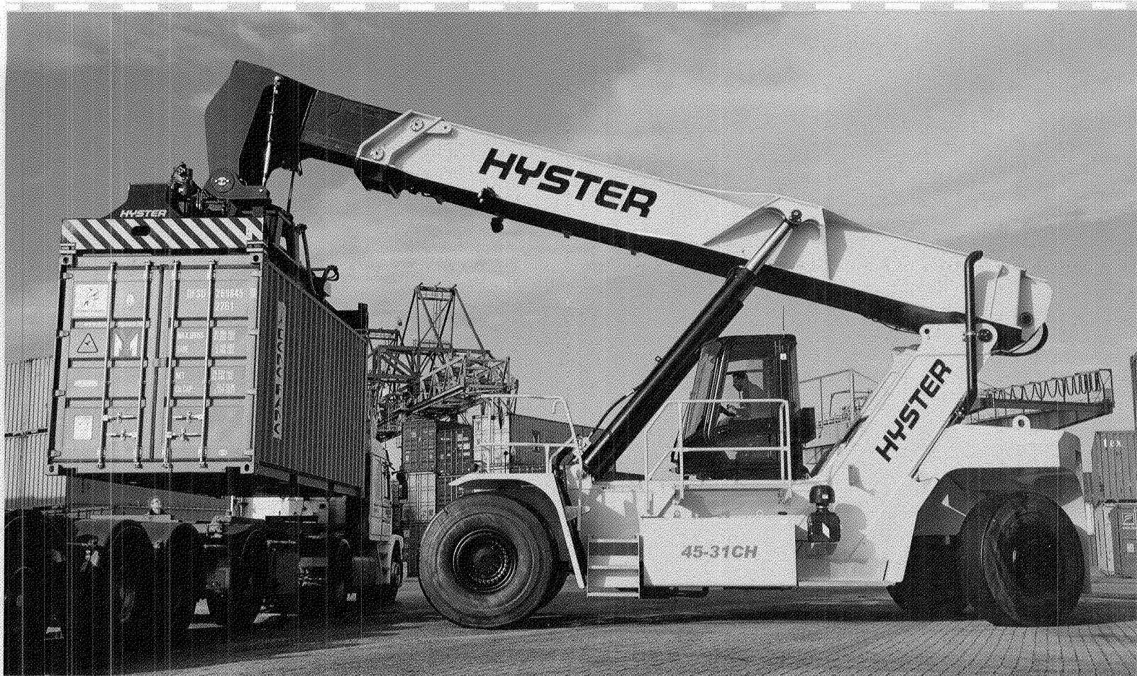
The new low emission, Tier 4 compliant, Hyster® RS45-31CH ReachStacker, for port and terminal applications, has a lifting capacity of up to 99,000 pounds and the capability to stack containers five high in the front row.
