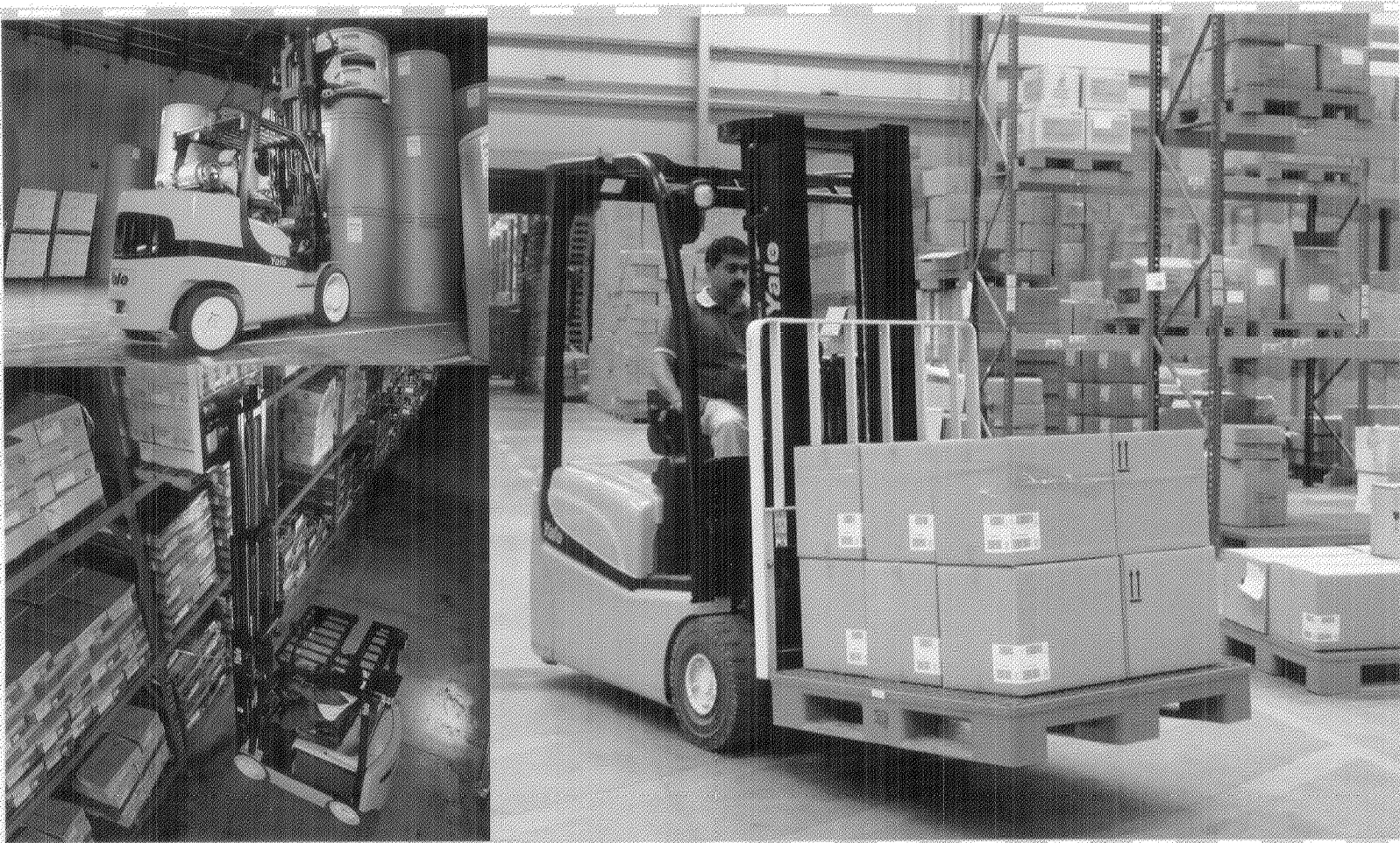
Clockwise from bottom left: One of Yale's new electric-rider lift truck series, the Yale® ERC-VA cushion tire series, has lifting capacities of 3,000 to 4,000 pounds. These trucks have been designed for overall productivity at lower costs; the four-wheel lift truck is shown here. This Yale® Veracitor® GC155VX internal combustion engine lift truck has a basic lifting capacity of 15,500 pounds and is shown here with a paper roll clamp attachment. Another series in Yale's new electric-rider lift truck series, the Yale® ERP-VT three-wheel pneumatic tire lift truck, has a zero-turn radius and a lifting capacity of 3,000 to 4,000 pounds.
