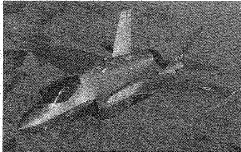
F-35A Conventional Takeoff and Landing (CTOL) Variant of the Joint Strike Fighter
