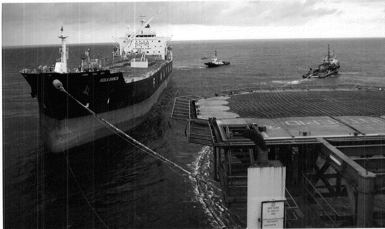
FPSO vessel "Rubicon Intrepid" engages the ocean-going tanker "Isola Bianca" in a crude oil offtake operation. Galoc Field, offshore NW Palawan
