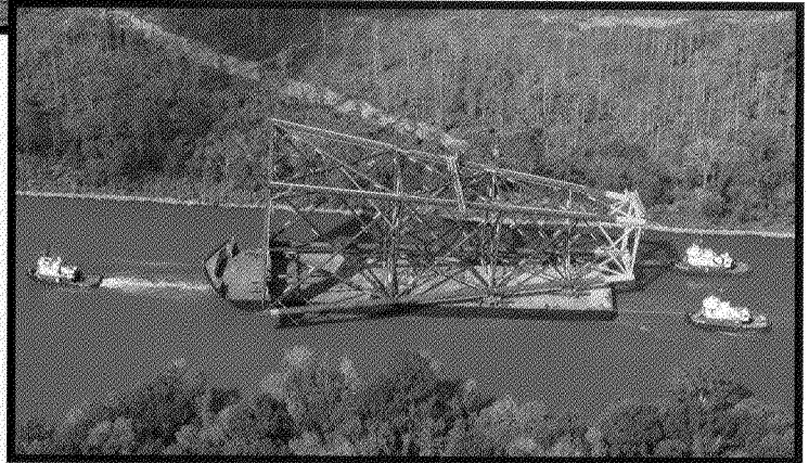
ATLANTA BRIDGE departing Central Louisiana with the base of an oil rig to be lifted off and put into position in the Gulf of Mexico
