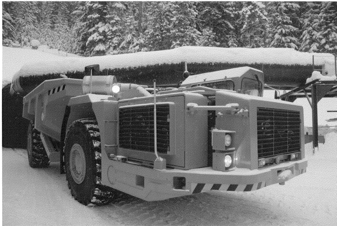
40-ton Sandvik haul truck situated outside portal to 14,000 ft. Montanore evaluation adit.
