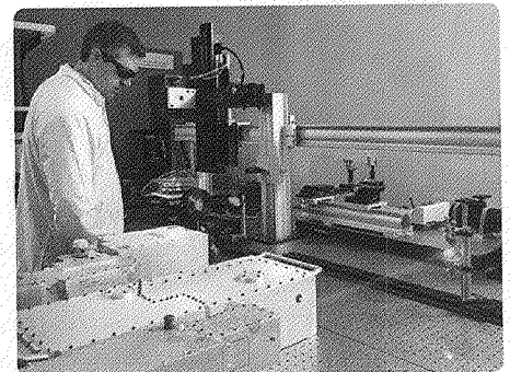
Engineers in Newport's Laser Applications Lab in Santa Clara perform experiments to determine the optimal Spectra-Physics laser configuration for their customers' materials processing applications.
