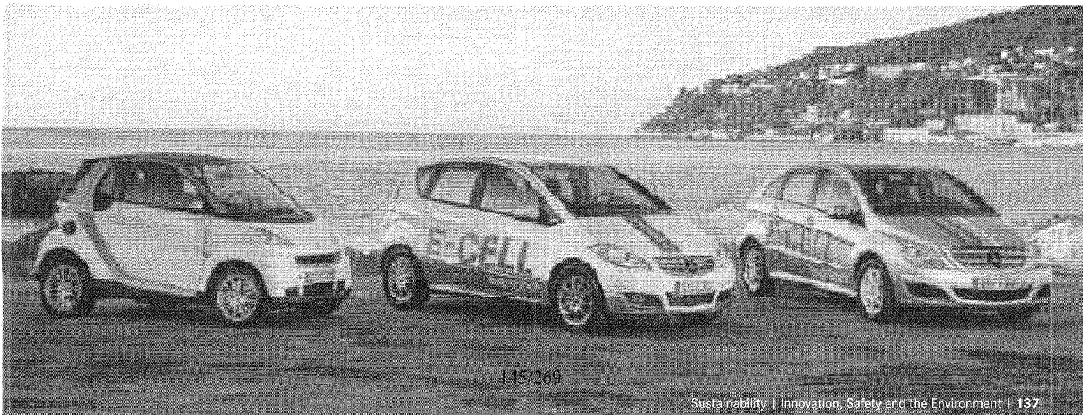
Electric vehicles with batteries and fuel cells: smart fortwo electric drive, A-Class E-CELL and B-Class F-CELL.
