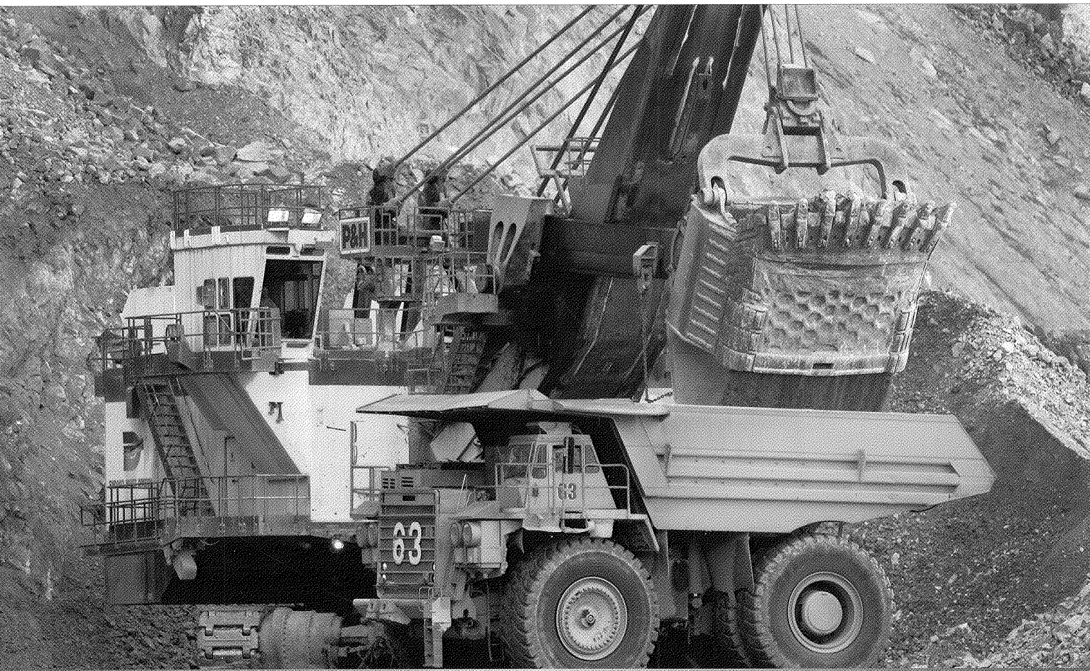
Electric shovel loading a haul truck at the Endako Mine
