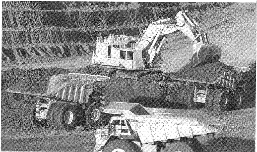
Right: At the Falkirk Mine in North Dakota, an electric shovel loads overburden into a fleet of Caterpillar end dump trucks to expose the coal for extraction.
