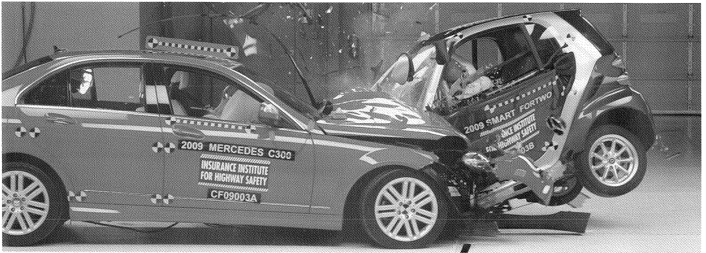
New crash tests performed by the Insurance Institute of Highway Safety (IIHS) in the U.S. demonstrate the influence of vehicle size and weight on safety in crashes. Smaller and lighter cars use less fuel, and therefore produce less CO 2 , but they can generally not protect people in crashes as efficiently as bigger, heavier vehicles. However, there are ways to enhance both fuel economy and safety. (Image credit: http://www.iihs.org ).
