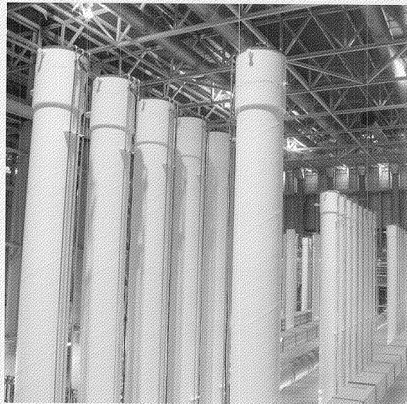
More than two dozen AC100 centrifuge machines are spinning in preparation for the Lead Cascade testing program.
