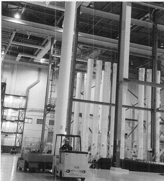
A 40-foot tall AC100 centrifuge machine moves slowly through the plant to the American Centrifuge demonstration area for installation.
