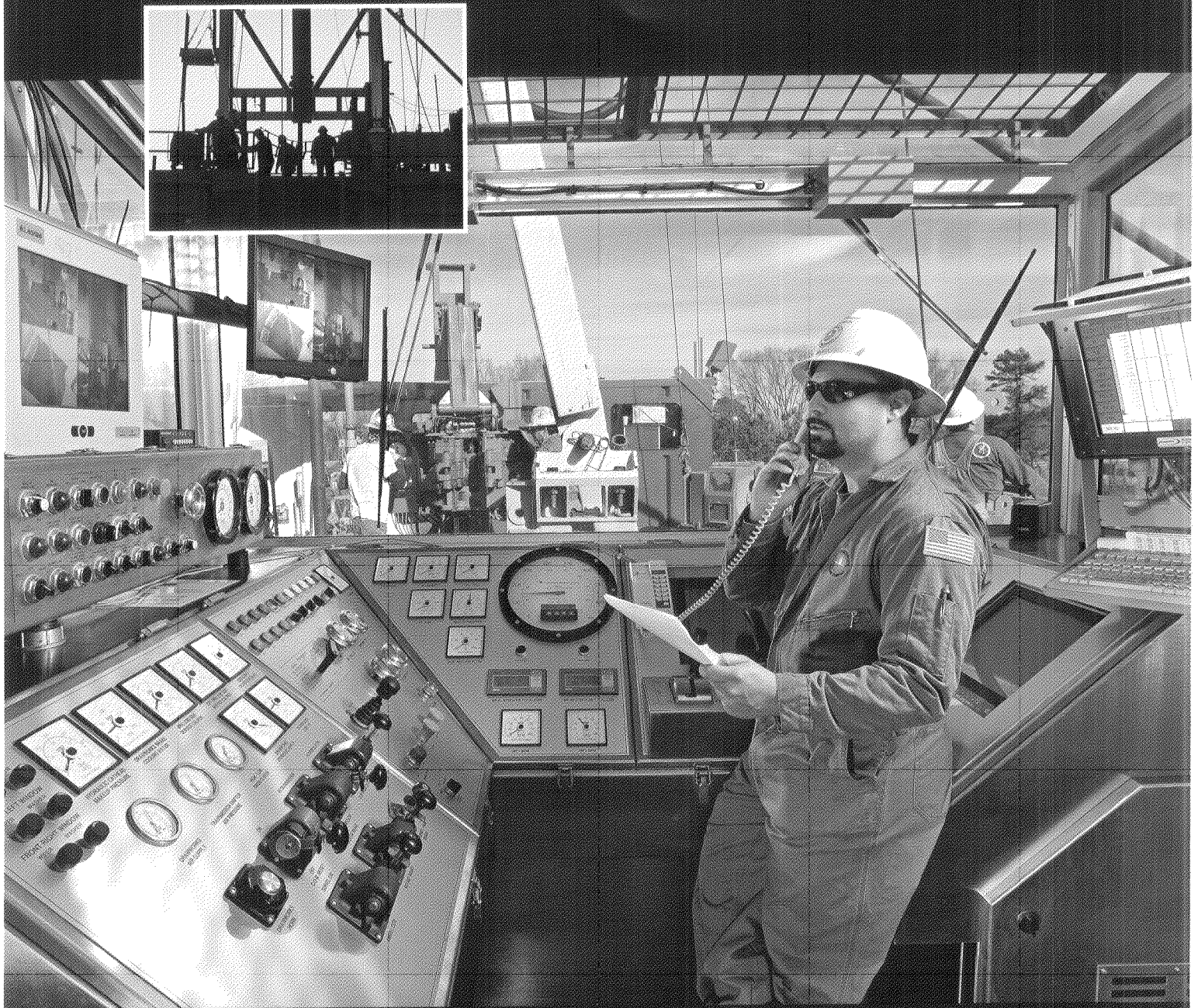
The Driller's Console on APEX® 1500 rigs offers a controlled environment and advanced technology systems to improve drilling efficiency.
