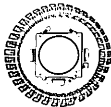
A Spire custom-made GaAs-based concentrator cell is relative to the size of a dime, above, and is enlarged to show detail, right.
