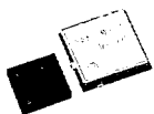
IC chip (left) and radio tuner module incorporating the IC chip (right)
