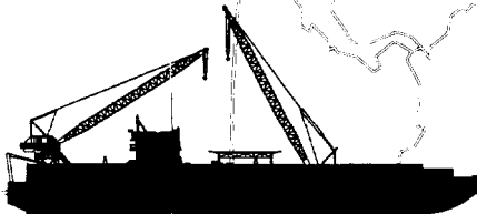
Lone Star Horizon 320' x 90', pipelay capacity of 39", jetting capabilities. Based out of Sabine Pass, Texas Marine Base.
