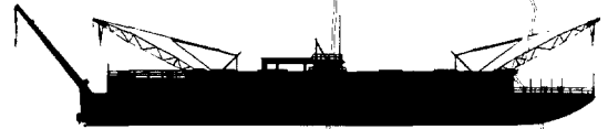
Gulf Horizon 350' x 71', pipelay capacity of 36", jetting capabilities. Based out of Sabine Pass, Texas Marine Base.
