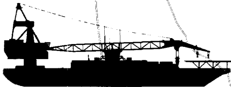
Pacific Horizon 350' x 100', lift capacity of 1,000 short tons. Based out of Sabine Pass, Texas Marine Base.
