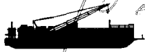
Cajun Horizon 140' x 40', pipelay/bury capacity of 12". Based out of Sabine Pass, Texas Marine Base.
