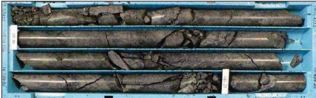
Figure 7.6: High Grade Covellite Breccia in Massive Pyrite - Hole FTMC1223 480.9 to 484.4 m
