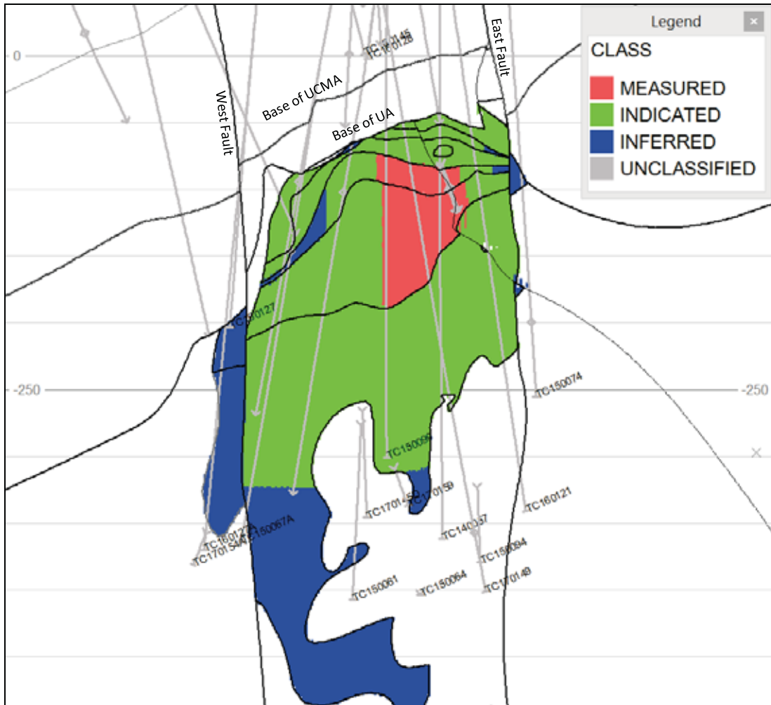
Figure 14.25: Cross-Section Showing SRK's Wireframe-Defined Mineral Resource Classification for the Timok Deposit, View North-Northwest
