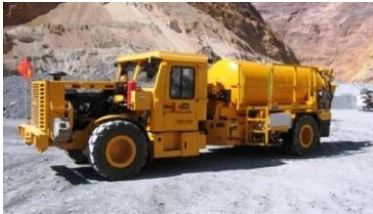
Figure 18-3: MacLean TM-3 Transmixer Tractor (Example)
