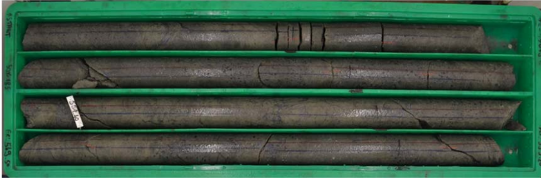
Figure 7-7: Massive Sulphide, Veins and Stockwork in More Coherent Andesitic Rock - Hole TC170150 at 549.5 to 5536.208 m
