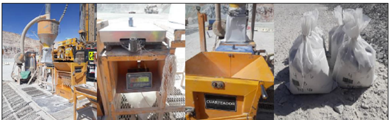
Figure 8-1: RC Sampling; A) Sample Collection; B) Weight control; C) Sample Splitting; D) A and B Samples
