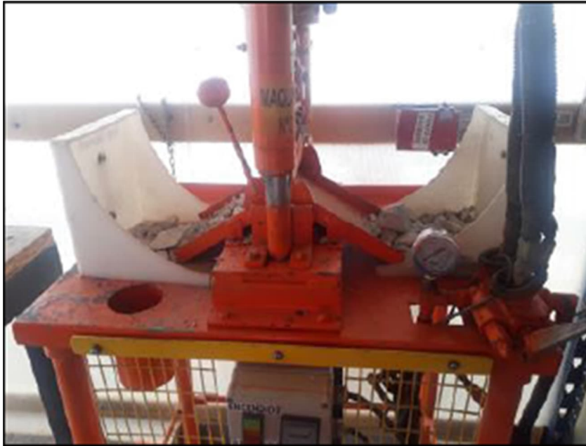
Figure 8-5: Hydraulic Guillotine for Core Cutting
