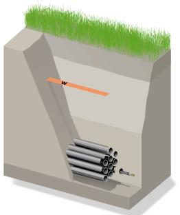
Level 3 is installing multiple conduits 42" below ground in its continuously upgradeable network. Ten to twelve 1½" conduits are grouped together. Fiber will initially be drawn through only one of the conduits, leaving the others for future expansion as technology changes, to meet customer demand and to provide Level 3 the flexibility to offer conduit to others.
