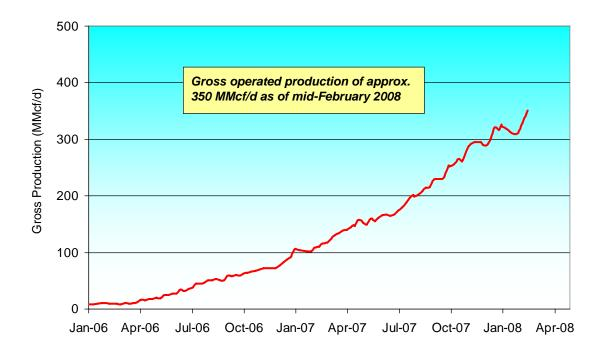
Southwestern has drilled and completed 116 wells with lateral lengths over 3,000 feet through February 19, 2008. Southwestern forecasts that the average gross ultimate recovery from wells with greater than 3,000 feet horizontal laterals to range from 2.0 to 2.5 Bcf per well with an average completed well cost of approximately \$3.0 million per well. Below are the results from these wells:
