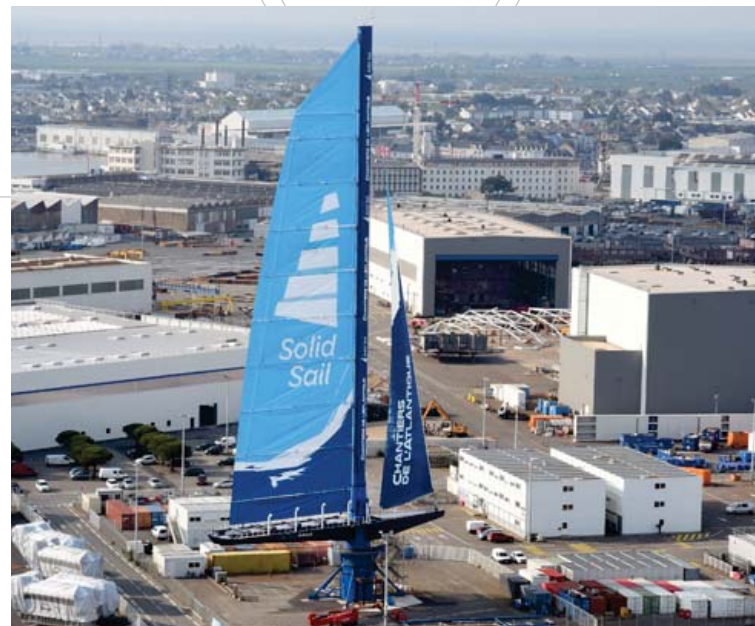
Hexcel supplies lightweight composites to Chantiers de l'Atlantique for its solid sail for cruise ships, a design to increase energy efficiency and lower environmental impact. ©Chantiers de l'Atlantique/Bernard Biger.
