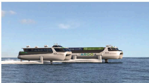
Hydrofoiling electric passenger ferry and micro containership powered by Valo's hydrofoil technology
