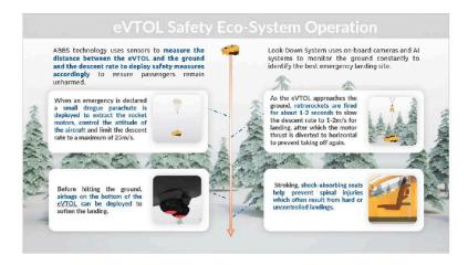
The "Zero Altitude - Zero Speed" EDAS system controls the descent rate to achieve a safe and soft landing.
