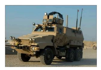
The high center of gravity results in instability and poor handling with roll-over accidents being quite frequent and the high vehicle presents a larger target for the enemy. The increased size and additional armor also made the vehicles very heavy with extremely high fuel consumption and almost no ability to move offroad for fear of getting bogged down in soft ground.
