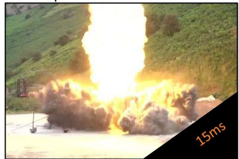
Linear Rocket Motors ignite, belly plate remains flat.
