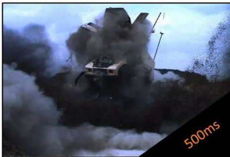
Belly plate deforms, breaking vehicle in half.
