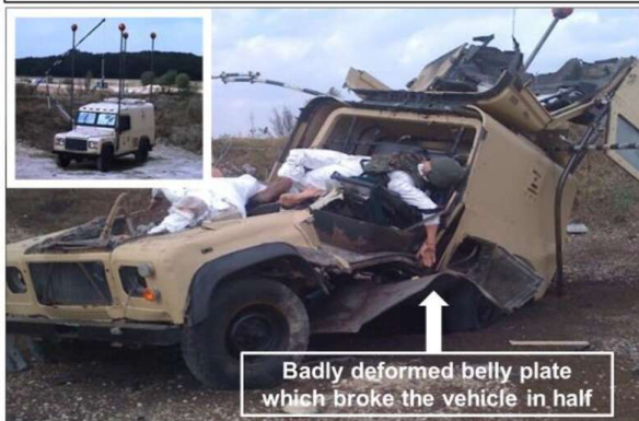
Result with Standard Belly Plate and 6kg Anti-Tank Mine
