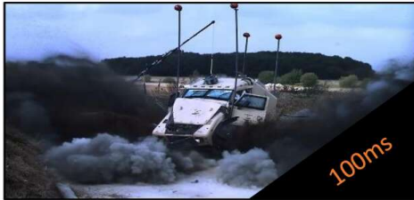
Belly plate deforms, breaking vehicle in half.
