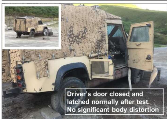
Result After 6kg Anti-tank Mine With ABBS System.
