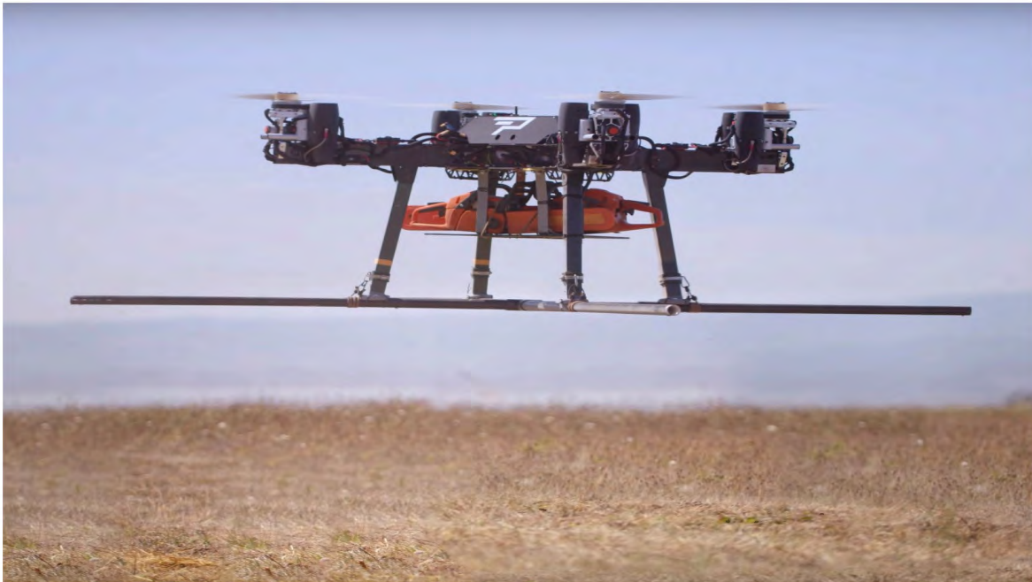
Prototype Parallel Hybrid Multirotor in flight with 18kg (40lbs) of payload
