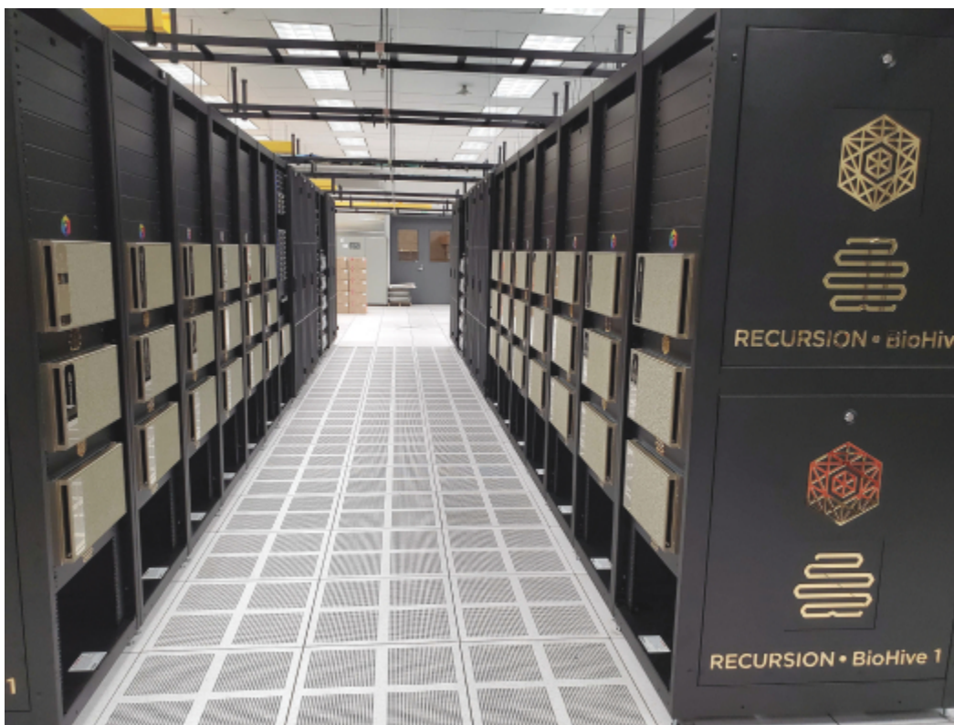
Figure 32. We believe BioHive-1 is one of the most powerful supercomputers dedicated wholly to drug discovery for a single company. BioHive-1 consists of 40 NVIDIA DGX A100 640GB nodes, which further expands our capability to rapidly improve ML models.
