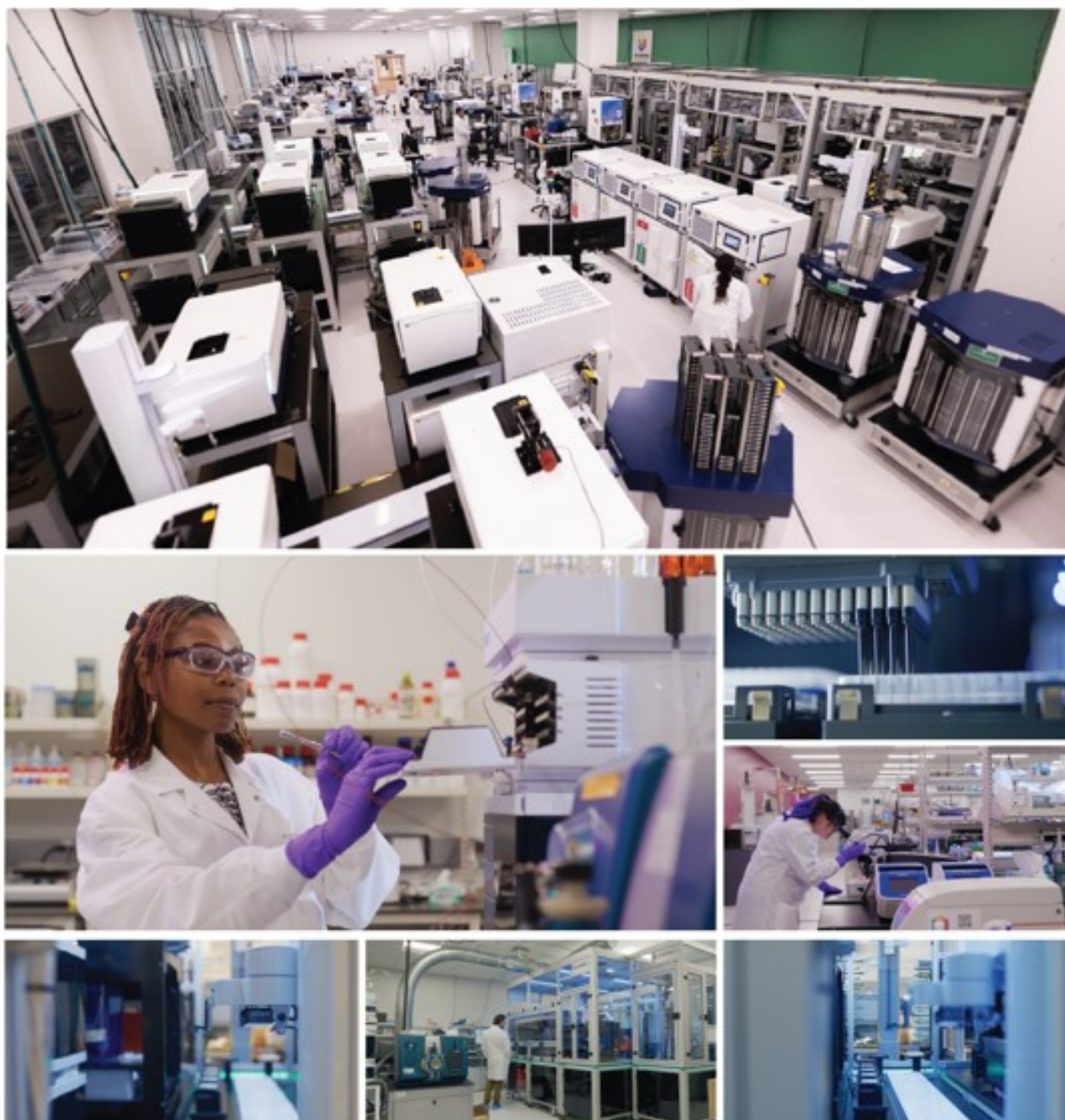
Figure 23. Our high-throughput automation platforms make our labs look more like sophisticated manufacturing facilities than biology R&D laboratories. Our high-throughput phenomics platform (top) can execute up to 2.2 million experiments each week with high quality to enable downstream analyses. We are increasingly automating many other of our assays at Recursion.
