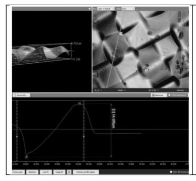
The image of the surface geometry of 30FWWHM micro facets is shown in the picture. This image was captured using a 3D Surface Profiler VK-X3000 from Keyence.
