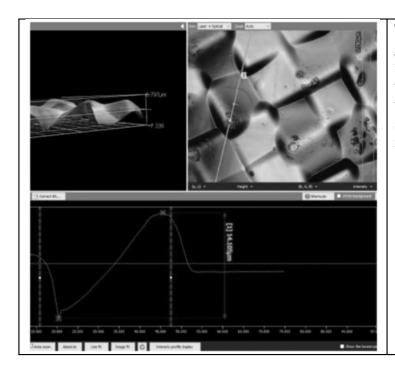
The image of the surface geometry of 30FWWHM micro facets is shown in the picture. This image was captured using a 3D Surface Profiler VK-X3000 from Keyence.
