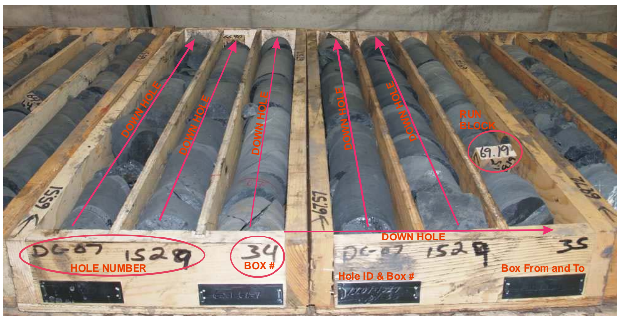
Figure 1: Typical layout and orientation of core as it is logged.
