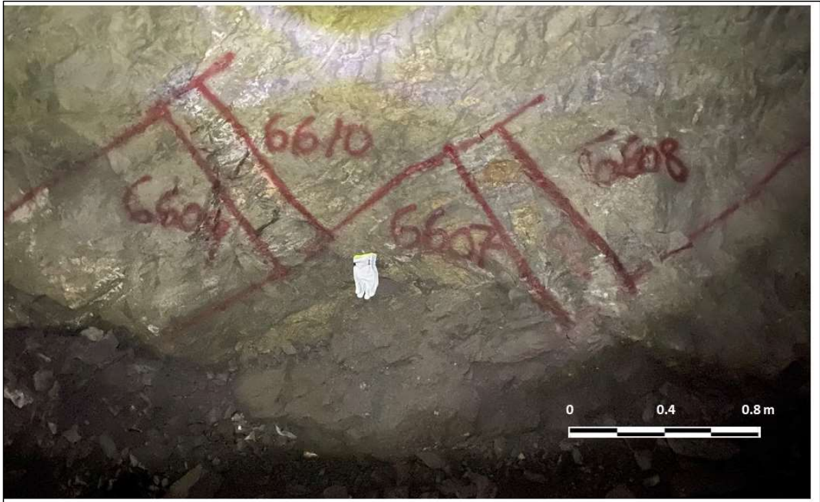
Figure 7-4: Marks Indicating Limits and Width of Samples
